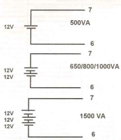
Use 12V batteries of maximum 32 AH for extending the backup time. Depending on the input DC voltage two batteries for 1000VA, two for 1000E and three for 1500VA are to be used.
