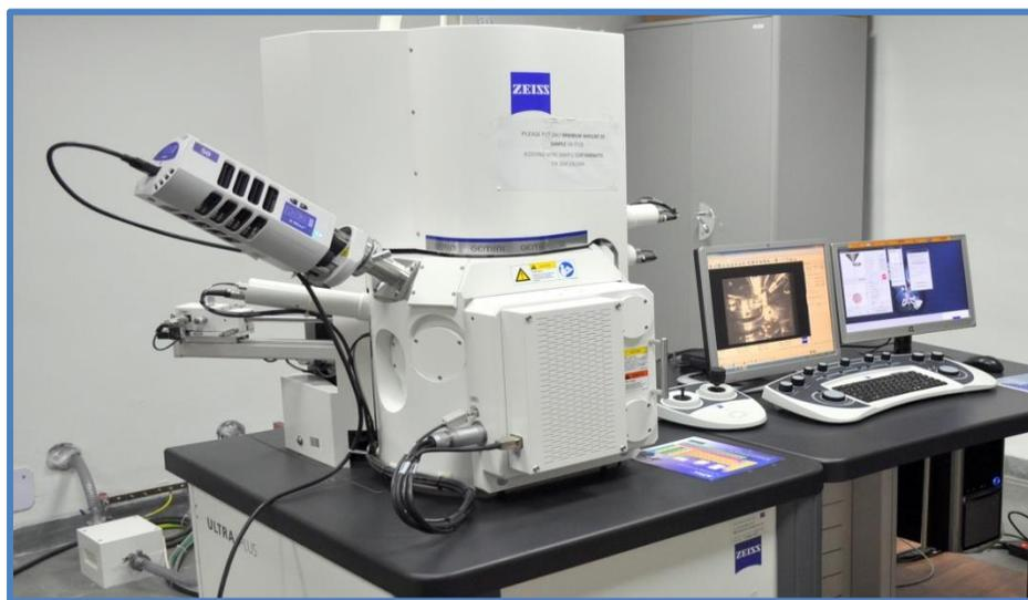
**Fig. 3.2: High Resolution Field Emission Scanning Electron Microscope**
