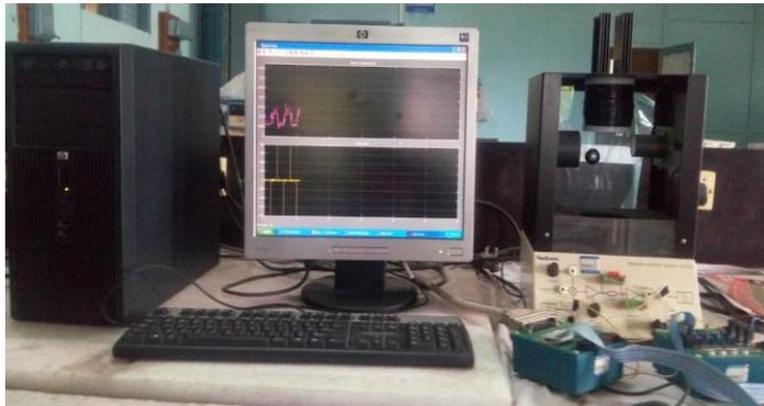
*Figure 6.1 Real time setup of Maglev system*
