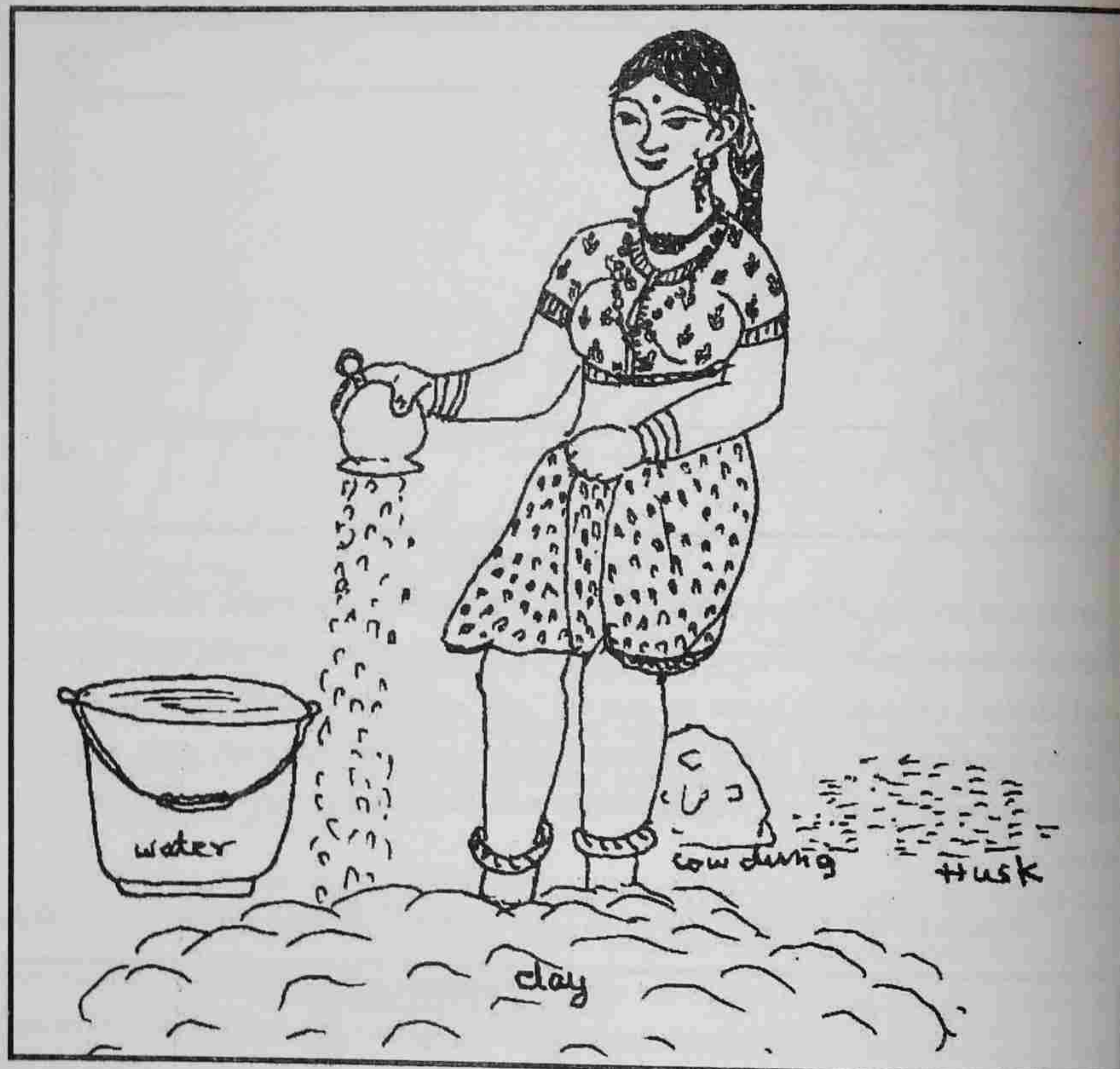
Method of preparing the mud by meshing
