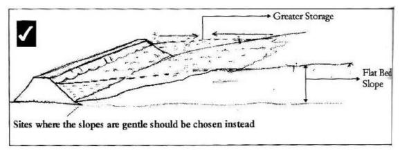
a. Slope of the Upstream Naala Bed: The bed slope should be relatively low (not
