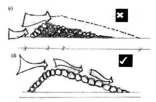
If small boulders are placed on the outer, particularly downstream face of the boulder check, water will exert pressure on the outer face (a); dislodge the small boulders there (b) and wash down the check (c). Thus large boulders must be placed on the outer face, particularly on the downstream side (d)
