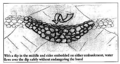
because the check will not be able to withstand the high velocity of water flow. However, on a drainage line with an overall high bed slope boulder checks can be constructed in sections where the local bed slope is less than 20%.
