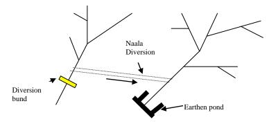
• When a valuable land is eroded by naala: - In that situation, naala can be diverted through artificial channel to near by drain. Caution should be taken while planning for diversion that the artificial channel does not erode any valuable land. If it is justified in terms of the cost benefit ratio than this type of plan may be considered for implementation
