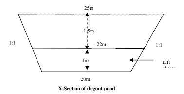
the dug out pond depends on the angle of repose, generally 1:1 side slope is provided in cutting section.
