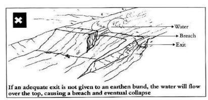
downstream face of the embankment. It, therefore, cuts channels on the downstream side and weakens the structure. Pitching and vegetative measures on the downstream side help keep the velocity of flow within the non-
