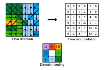
Figure 11:- D8 algorithm for calculation of flow direction
