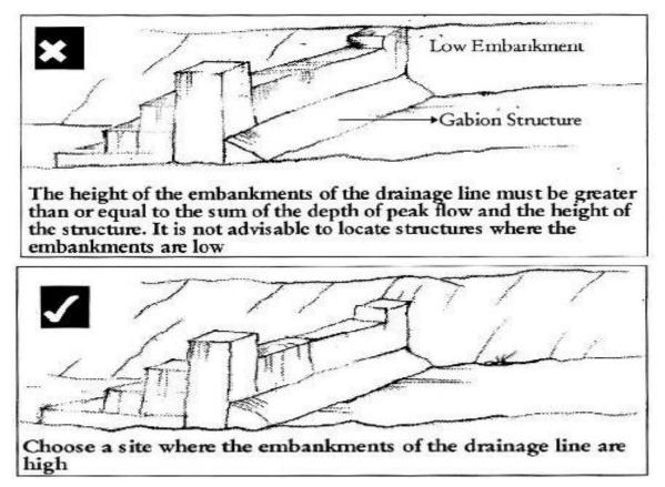
equal the sum of the depth of peak flow in the stream and the designed height of the structure. For example, if the height of the embankments is 6 m and the depth of peak flow is 4 m, then the height of the gabian must not exceed 2 m to prevent the water from jumping over the sides. Hence, observation of the peak flows is imperative before a gabian structure is planned.
