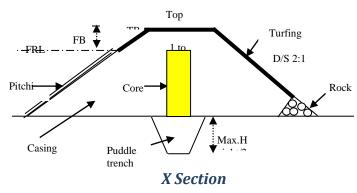
must be very carefully determined. The precise upstream and downstream slopes of the structure depend on the angle of repose and erodability of the materials used in the outermost faces. Through experience it has been found that for a stable earthen structure, the upstream slope should range from 2:1 to 4:1. The downstream slope should range from 2:1 to 3:1. In general 2:1 slope is provided on the upstream and downstream of the structure.
