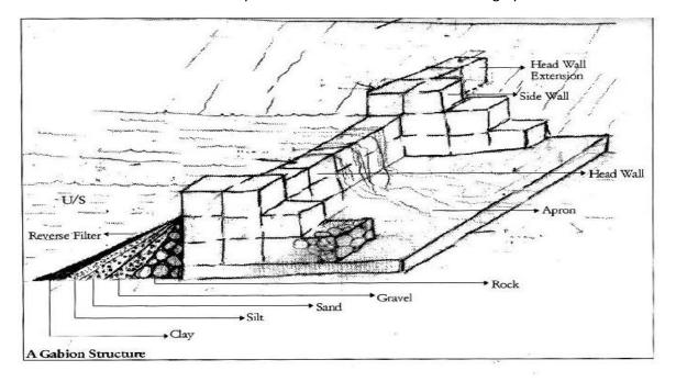
embankments. In this module, we will first describe Gabians across drainage lines in great detail. In the end, we provide a short note on Gabians built along embankments.
