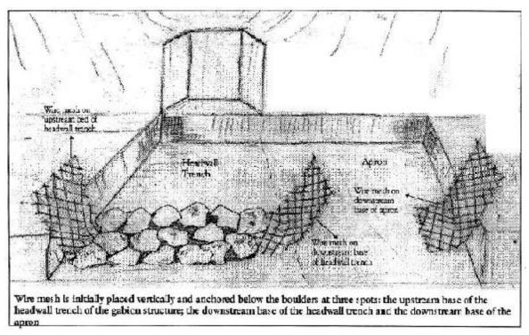
Everywhere, 0.15 m of the wire mesh is folded along the bed of the trench so that the mesh can be embedded under the boulders. After that the trench is filled with boulders up to ground level. Then the wire mesh is laid over the entire surface and tied to that mesh, which has been embedded under the boulders. The headwall as well as the sidewalls should be constructed as boxes of 1 to 2 m length and 1 m height.
