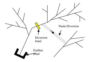
• When a site fulfills all the points of ideal site selection criteria, with an exception that the catchment is not enough for planned storage capacity of water harvesting structure: - In that situation, nearby naala (as per requirement) can be diverted through an artificial
