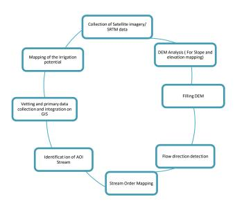
Figure 12:- Process flow for stream network analysis
