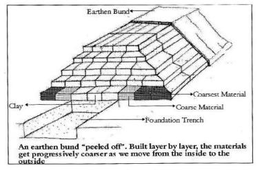
Where there is an easy availability of clay, a heart type of structure may be made. A thicker wall of clay can be raised by laying, wetting and ramming. After the cut off trench has been filled, the structure comes up in horizontal layers. All sections of the structure must be raised together. In a core wall type, the puddle core wall and the shell must be simultaneously raised. In the heart type, both the hearting and the
