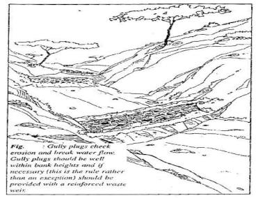
If the slope is 10% or more, keep the horizontal distance between two boulder checks as 10 m. In case the slope is less than 10%, then increase the distance between the boulder checks, depending on the flatness of the slope. Thus, for instance, if the slope is 5%, the distance should be 20 m; if slope is 2%, the distance should be 50 m. Even if the slope is less than 2%, do not increase the distance beyond 50 m, which is the maximum distance we have fixed.
