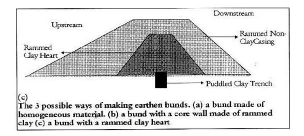
**Heart type**: Where clay is available easily and in large quantities, it is possible to construct the heart of the bund with wetted and rammed clay, and providing a casing of coarser soils to protect it. In situations where pure clay is not available, it is still possible to make a farm pond using finer and clayey soils for the heart of the structure and graduating to coarser soils in the casing.
