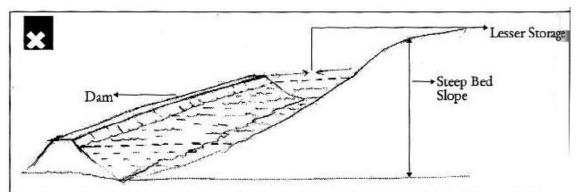
Structures should not be built where the slope of the drainage line is high. This results in lesser volume of storage (other factors remaining constant) and may breach the structure.
