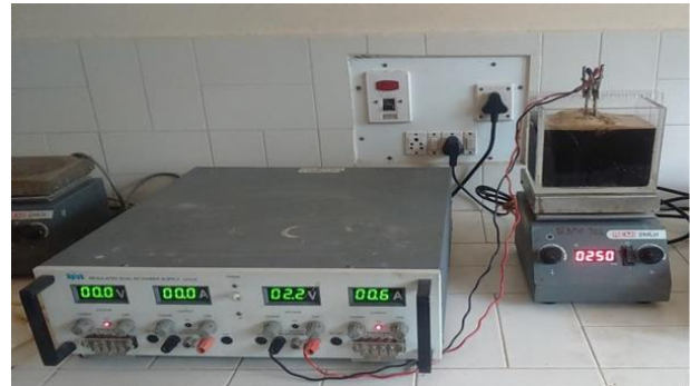
Fig 2 Experimental set up of electrocoagulation treatment in a lab scale
