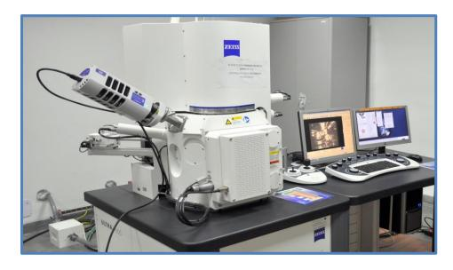
Fig. 3.2: High Resolution Field Emission Scanning Electron Microscope
