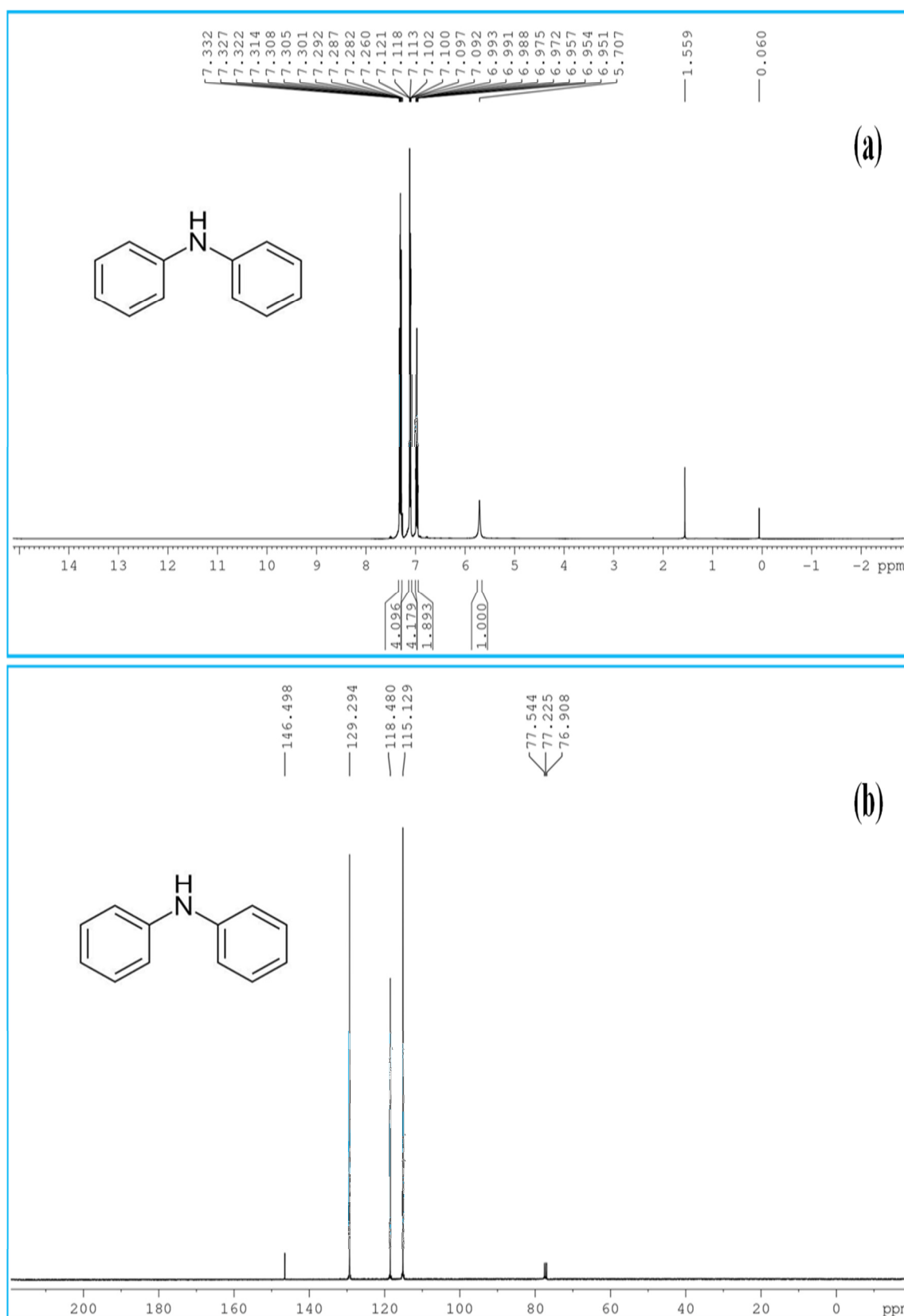
Fig. 4.8 : a) ^1\text{H} NMR and b) ^{13}\text{C} NMR spectra of Diphenylamine. In \text{CDCl}_3
