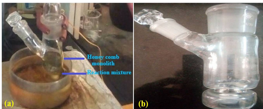
Fig.4.5 : Photographs of a) the reaction mixture and coated honeycomb catalyst. b) Specially designed reaction flask (reactor) for the C-N coupling reaction.
