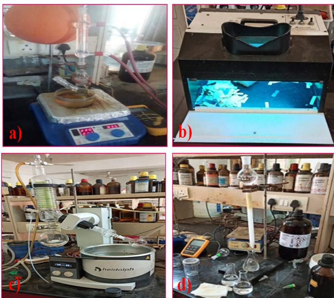
Fig.4.2 Photograph of a) C-N coupling reaction setup b) UV cabinet c) Rota evaporator d) Celite bed.
