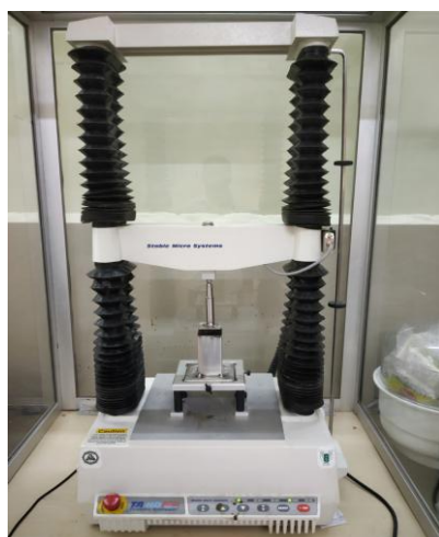
Plate 3.3: Texture analyser and fixture probe
