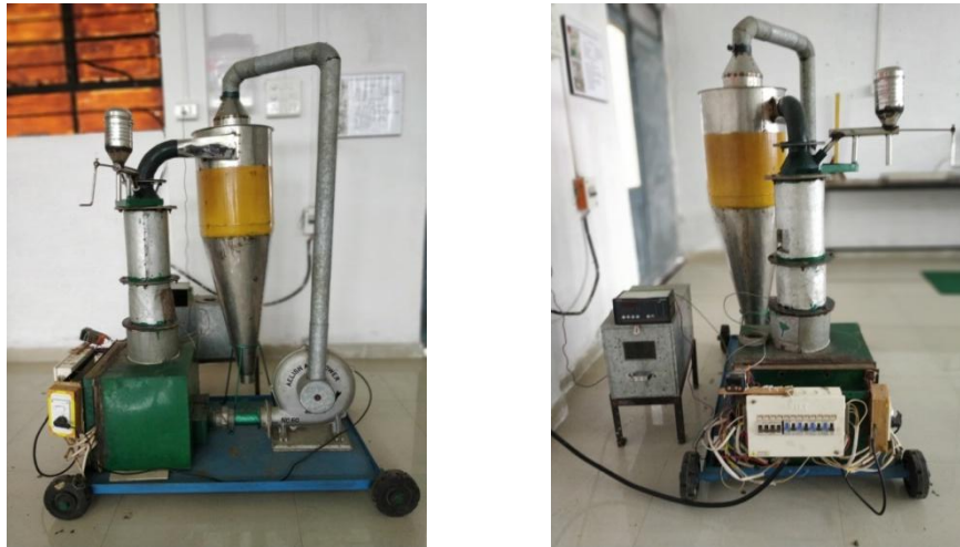
Plate 3.2: Semi-automated multigrain continuous hot air puffing system
