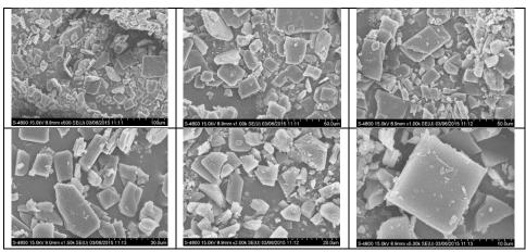
Figure 2.24(a): FE-SEM images of ENCu(II) complex at different magnifications
