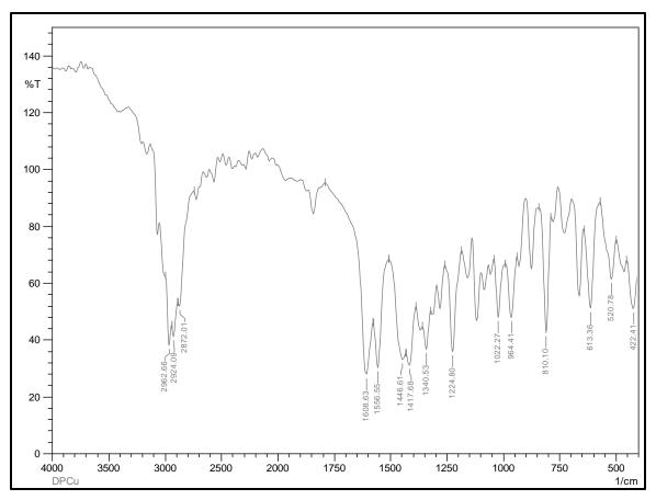
Figure. 3.13: FT-IR spectrum of DPCu(II) complex
