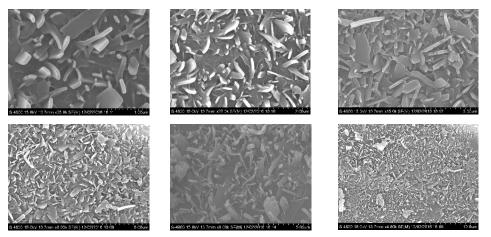
Figure 4.20(a): FE-SEM images of PHMn(III) complex at different magnifications
