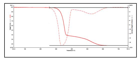
Figure 3.26: TGA curve of DPCu(II) complex
