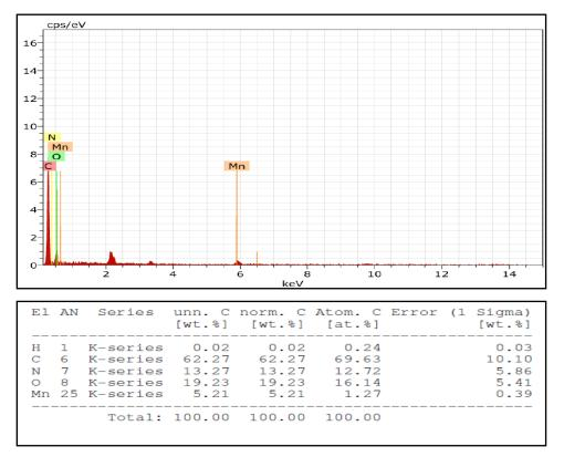
Figure 4.20(b): EDX analysis of PHMn(III) complex
