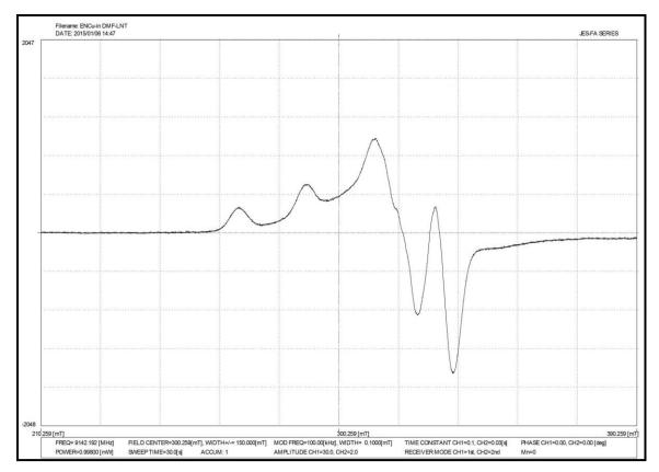
Figure 2.20: X-band ESR spectrum of ENCu(II) complex
