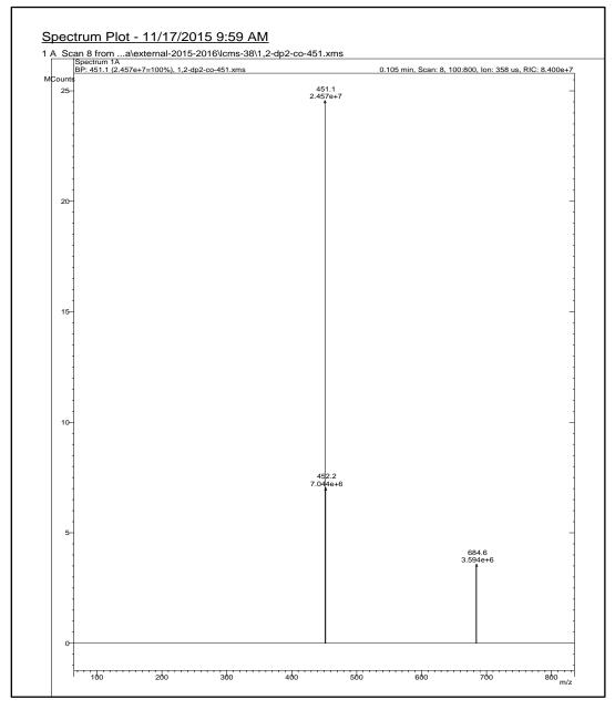
Figure 5.16: LC-MS spectrum of 1,2-DPCo(II) complex
