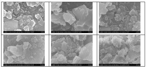
Figure 2.21(a): FE-SEM images of ENMn(III) complex at different magnifications
