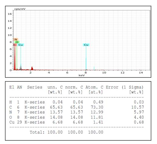
Figure 4.23(b): EDX analysis of PHCu(II) complex
