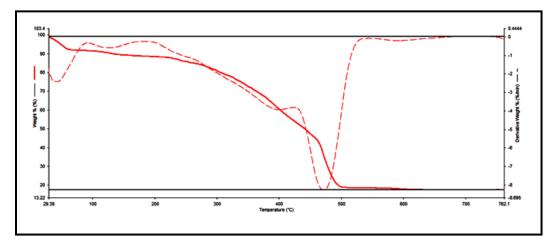
Figure.3. 23: TGA curve of DPMn(III) complex
