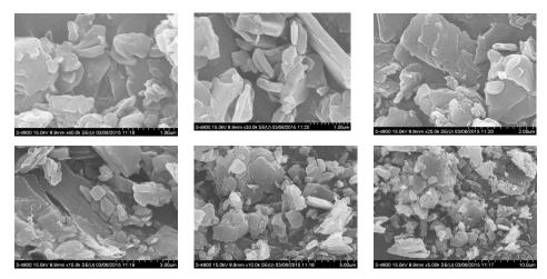
Figure 3.21(a): FE-SEM images of DPNi(II) complex at different magnifications
