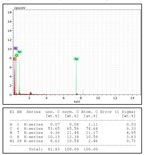
Figure 5.22 (b): EDX analysis of 1,2-DPNi(II) complex
