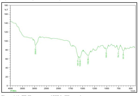
Figure 4.10: FT-IR spectrum of PHMn(III) complex
