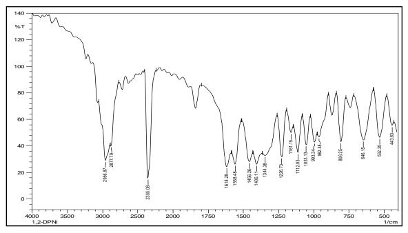
Figure 5.12: FT-IR spectrum of 1,2-DPNi(II) complex
