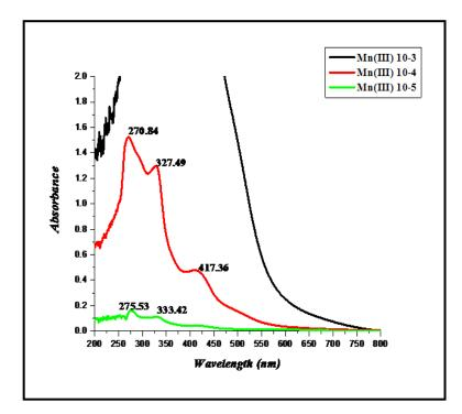
Figure 2.6: UV-Visible spectrum of ENMn(III) complex
