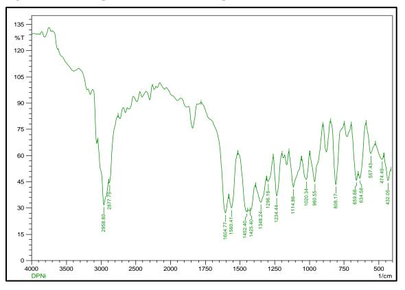
Figure 3.12: FT-IR spectrum of DPNi(II) complex
