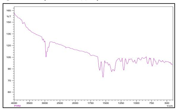
Figure. 4.12: FT-IR spectrum of PHNi(II) complex
