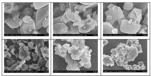
Figure 5.22(a): FE-SEM images of 1,2-DPNi(II) complex at different magnifications
