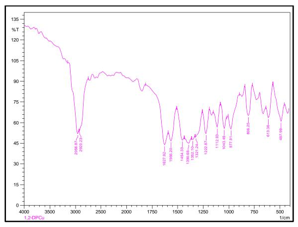
Figure 5.13: FT-IR spectrum of 1,2-DPCu(II) complex
