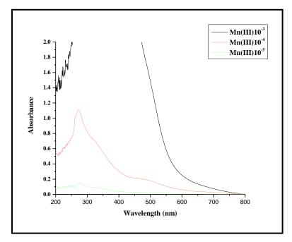
Figure 3.5: UV-Visible spectrum of DPMn(III) complex
