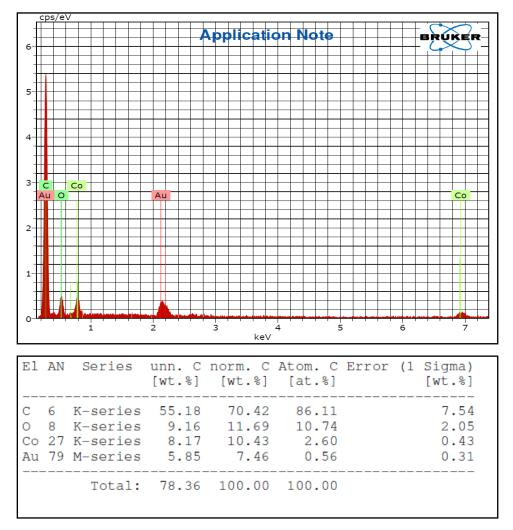
Figure 4.21(b): EDX analysis of PHCo(II) complex
