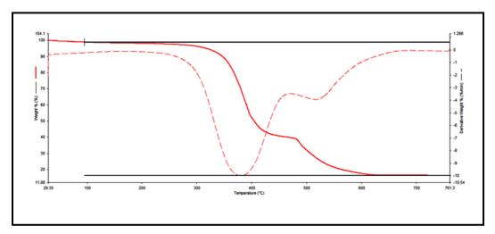
Figure 3.25: TGA curve of DPNi(II) complex
