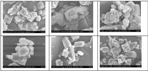
Figure 5.21(a): FE-SEM images of 1,2-DPCo(II) complex at different magnifications
