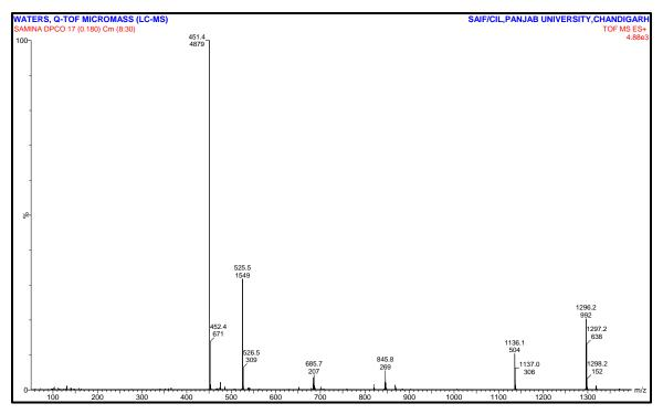
Figure 3.16: LC-MS spectrum of DPCo(II) complex
