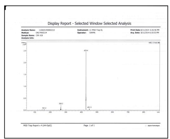
Figure 4.14: LC-MS spectrum of PH ligand
