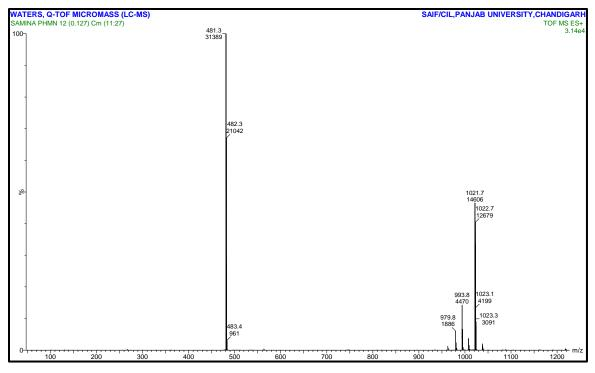
Figure 4.15: LC-MS spectrum of PHMn(III) complex
