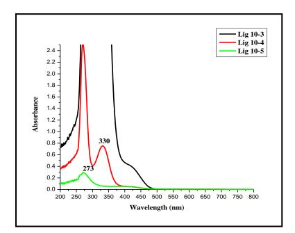
Figure 3.4: UV- Visible spectrum of DP ligand
