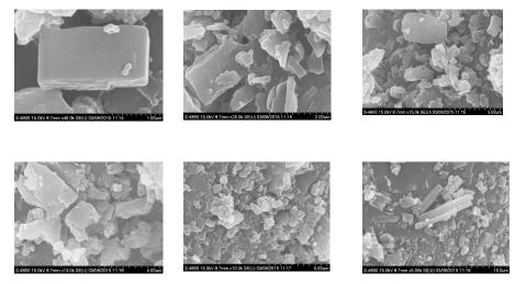
Figure 3.20(a): FE-SEM images of DPMn(III) complex at different magnifications
