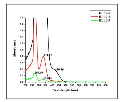
Figure 5.4: UV- Visible spectrum of 1,2-DP ligand
