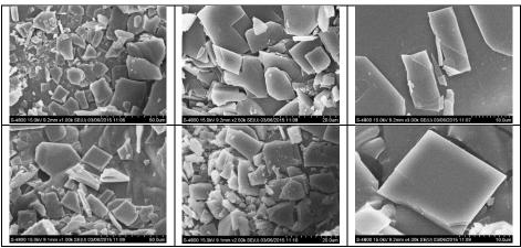
Figure 2.23(a): FE-SEM images of ENNi(II) complex at different magnifications
