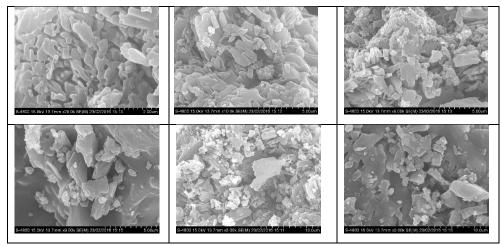
Figure 5.20(a): FE-SEM images of 1,2-DPMn(III) complex at different magnifications
