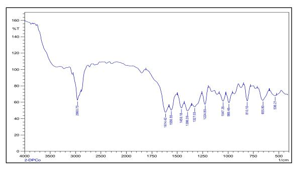
Figure 5.11: FT-IR spectrum of 1,2-DPCo(II) complex
