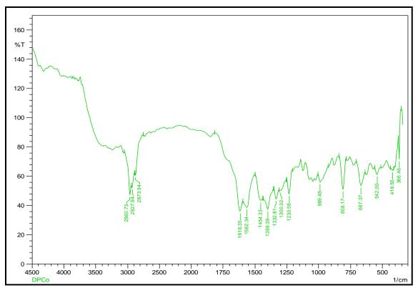
Figure 3.11: FT-IR spectrum of DPCo(II) complex
