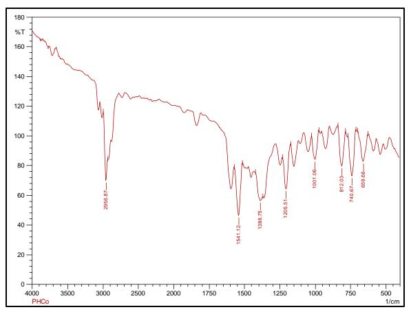
Figure 4.11: FT-IR spectrum of PHCo(II) complex
