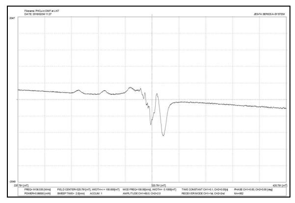
Figure 4.19: X-band ESR spectrum of PHCu(II) complex
