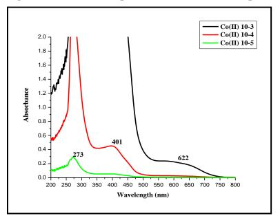
Figure 3.6: UV-Visible spectrum of DPCo(II) complex
