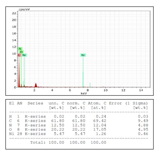
Figure 4.22(b): EDX analysis of PHNi(II) complex
