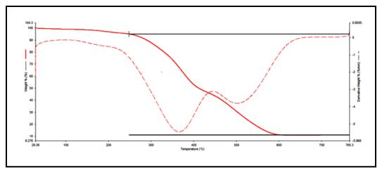
Figure 3.24: TGA curve of DPCo(II) complex
