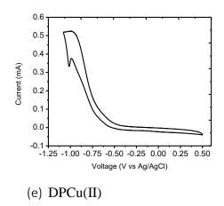
Figure 3.27 Cyclic voltammograms of (a) DP ligand; (b) DPMn(III); (c) DPCo(II); (d) DPNi(II); and (e) DPCu(II) complexes at room temperature in DMF solution containing 0.1 M TBAP as electrolyte at scan rate of 100 mVs<sup>-1</sup>.
