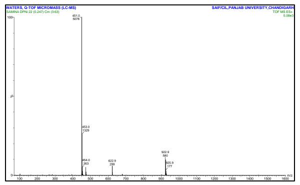
Figure 3.17: LC-MS spectrum of DPNi(II) complex
