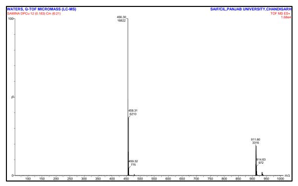
Figure 3.18: LC-MS spectrum of DPCu(II) complex
