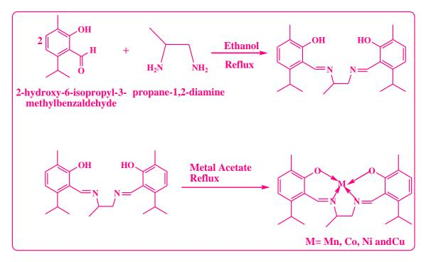
Figure 5.1: Synthesis of 1,2-DP ligand and its metal complexes.
