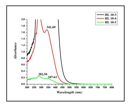
Figure 4.4: UV- Visible spectrum of PH ligand
