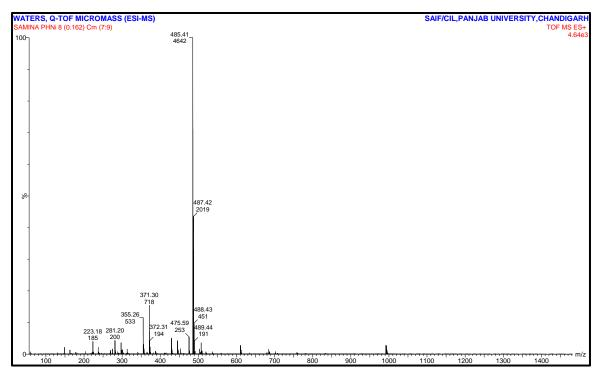
Figure 4.17: LC-MS spectrum of PHNi(II) complex
