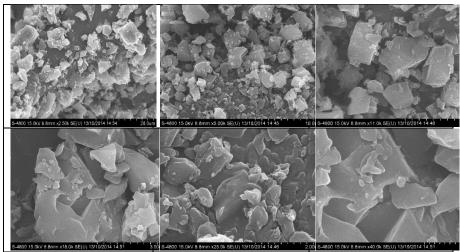
Figure 2.22(a): FE-SEM images of ENCo(II) complex at different magnifications
