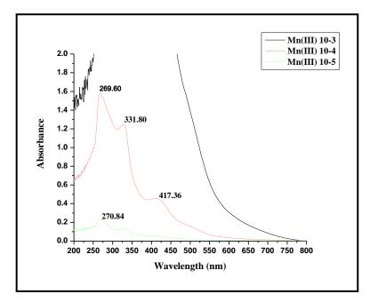
Figure 5.5: UV-Visible spectrum of 1,2- DPMn(III) complex
