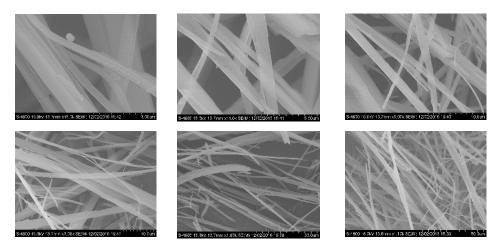
Figure 4.23(a): FE-SEM images of PHCu(II) complex at different magnifications
