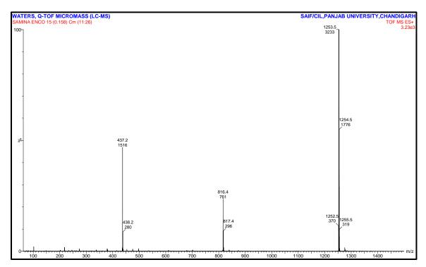
Figure 2.17: LC-MS spectrum of ENCo(II) complex
