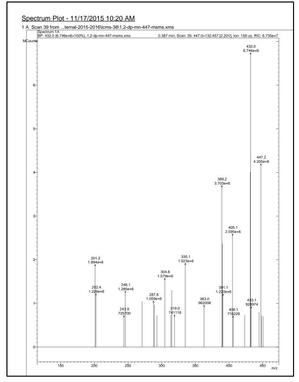
Figure 5.15: LC-MS spectrum of 1,2-DPMn(III) complex
