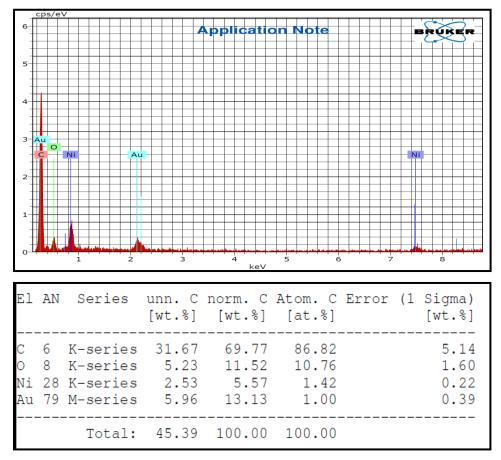
Figure 3.21(b): EDX analysis of DPNi(II) complex
