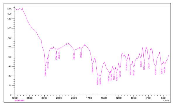
Figure 5.10: FT-IR spectrum of 1,2-DPMn(III) complex
