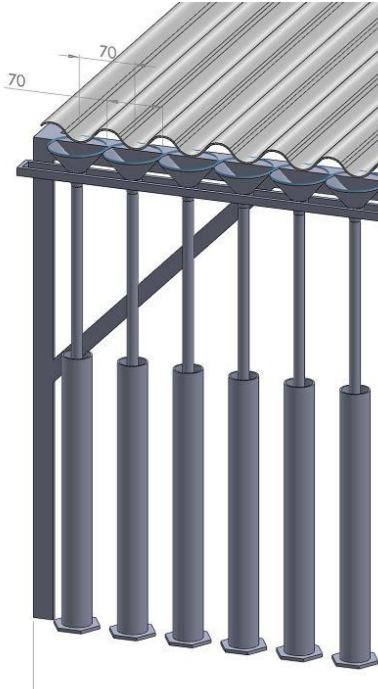
Fig. 8 Specifications of the patternator sheet
