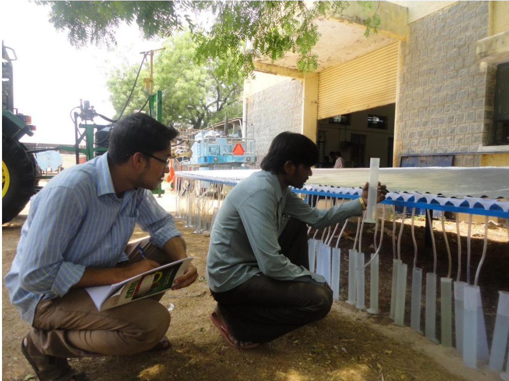
Plate 7 Measurement of volume of liquid collected in measuring jar
