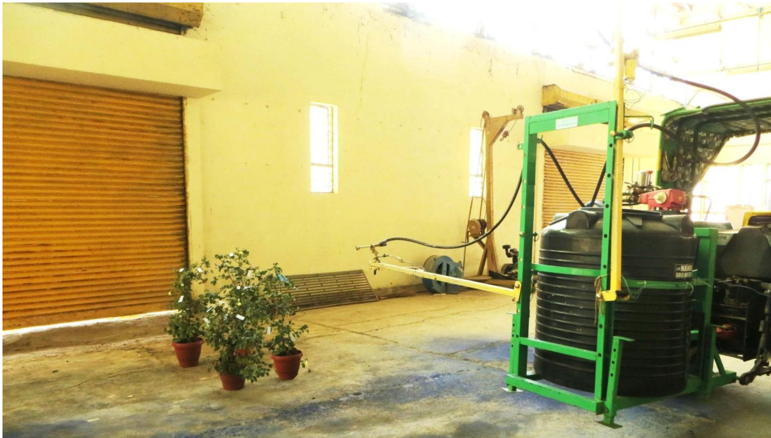
Plate 5 Arrangement of actual plant for evaluation of the sprayer in laboratory
