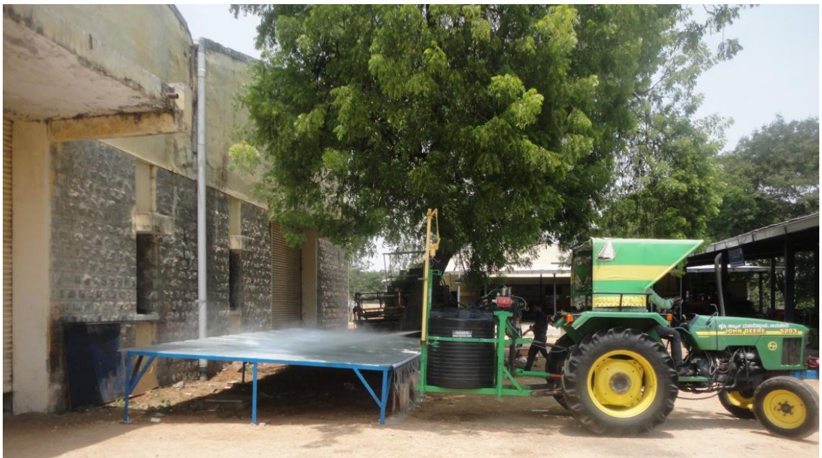
Plate 6 Evaluation of volumetric distribution of sprayer in patternator
