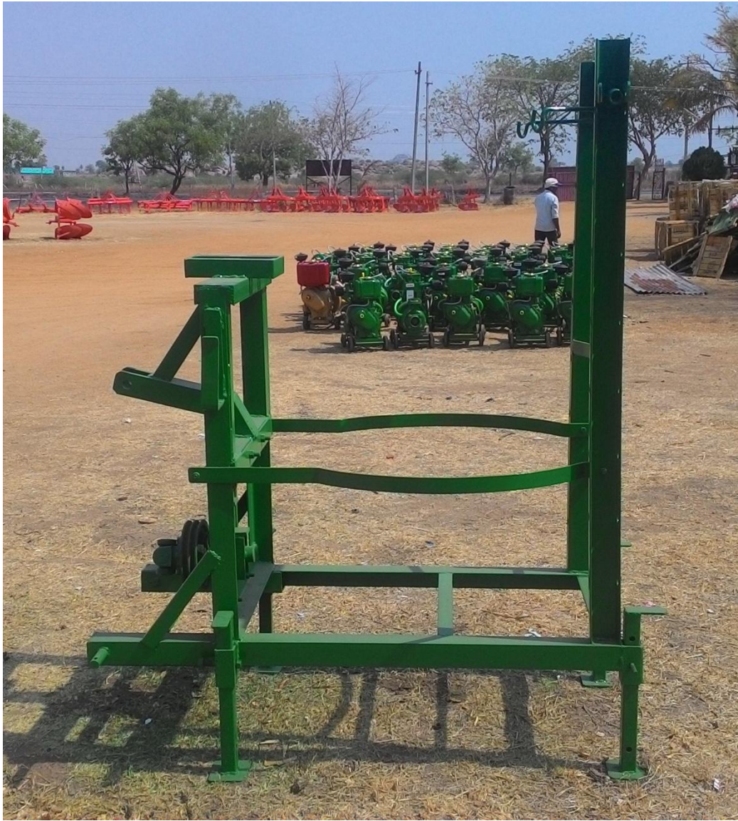
Plate 4 Prototype of the developed frame structure for automatic gun sprayer
